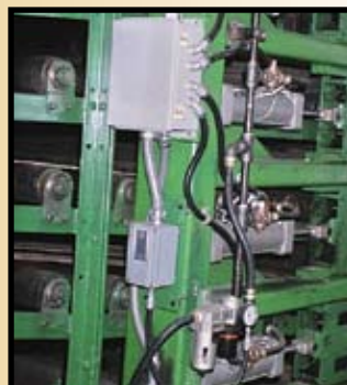
All electrical devices pre-wired to junction box
