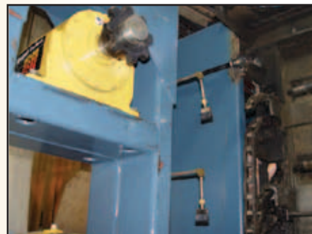
Gearbox and sprocket, shown with optional chain lubrication brushes
