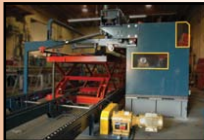
Dryer infeed with accumulator
