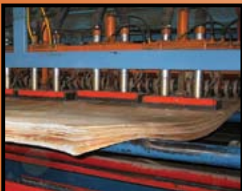
Accumulator supporting veneer during load change.
