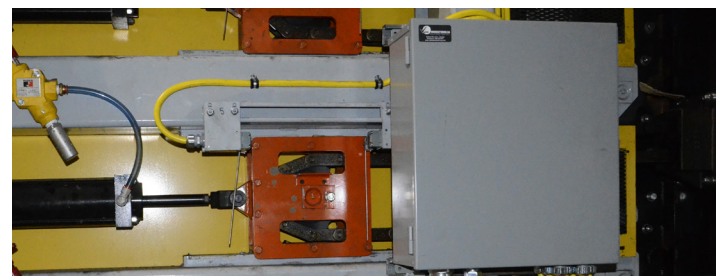
All electrical devices pre-wired to junction box
