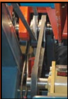
Polychain belt drive – quieter than roller chain
