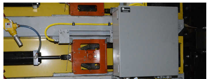
All electrical devices pre-wired to junction box
