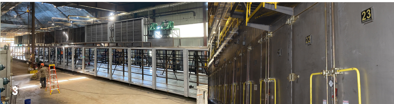
Worlds Longest Veneer Dryer: Roseburg, Coquille over 205 Ft (2,463") in length.
