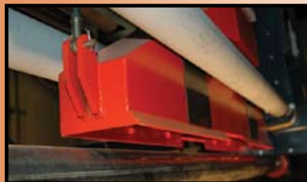
Vacuum box (orange) with powered rolls (gray)
