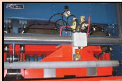
Vacuum head with Ross pneumatic valves and Banner photo eye wired to junction box
