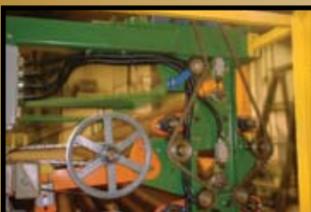
Continuous Serpentine Chain Drive
