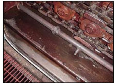
Perimeter water pipe and spray nozzle
