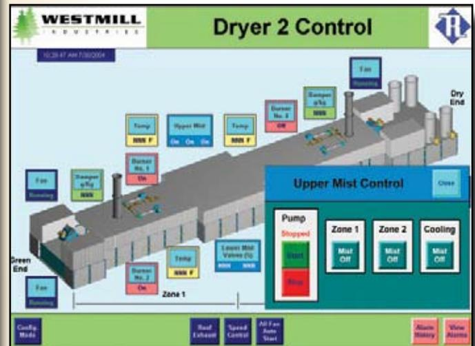
**The Humidity Monitoring and Spray Control System monitors the humidity inside the veneer drying chamber and can be operated as a stand-alone system.**
