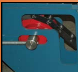
All idler sprockets come with relubricatable pins.
