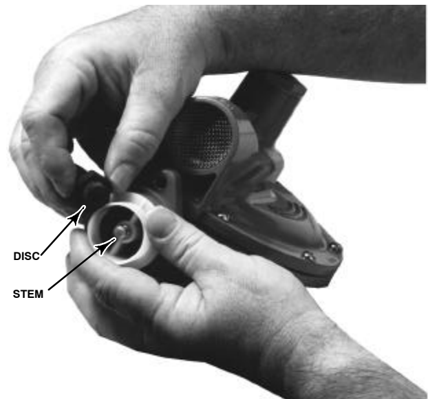
Figure 2. Reassembling Disc and Stem
