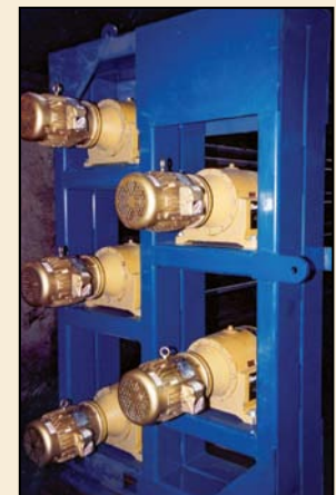
Our veneer dryer drive tower features independent deck drives.
